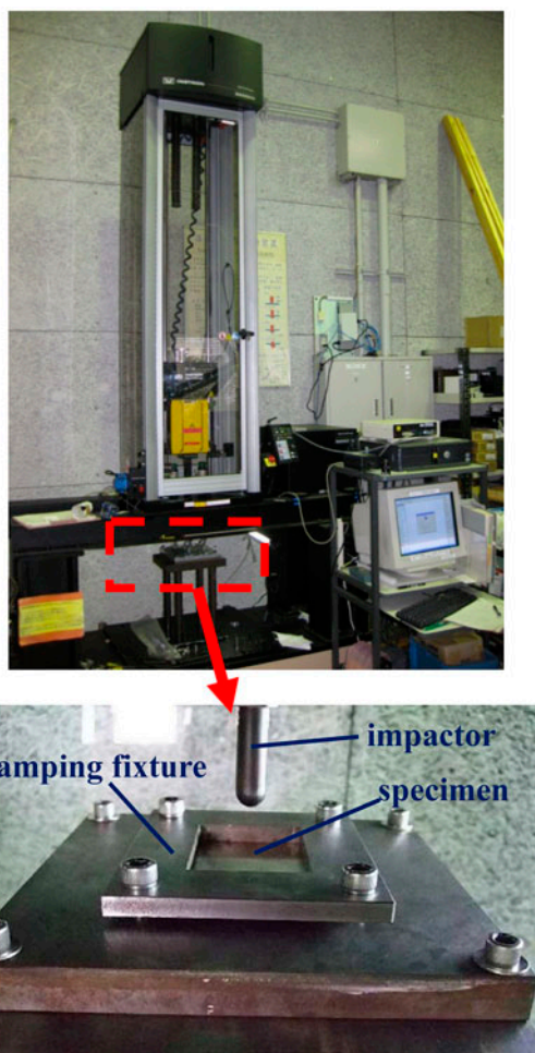
Figure 2. Drop-weight impact test apparatus of TMC specimens.
