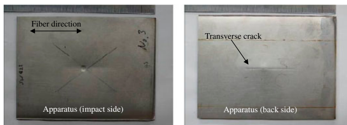
Figure 5. Impact damage of SiC/Ti with clad layers subjected to 45 J impact.
